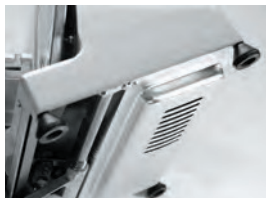
Air cooled engine protected by metal cover
